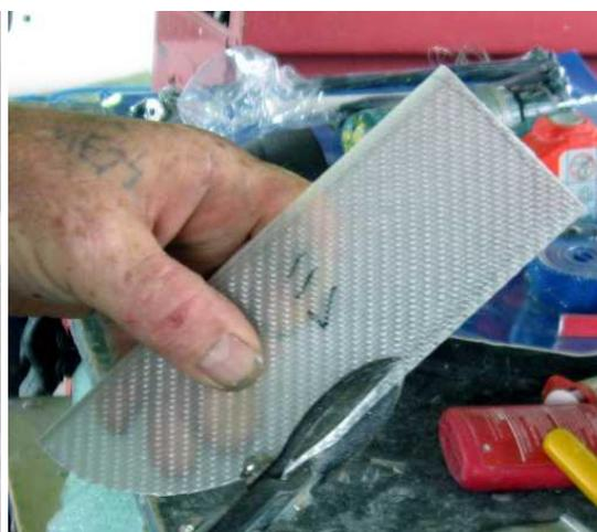
cut to size. Take the length of glass fibre sheet with the curved edge, hold it against the rear of the duct inlet with the curve towards the top rear of the duct and mark around the bottom of the duct then cut to shape as shown above.
