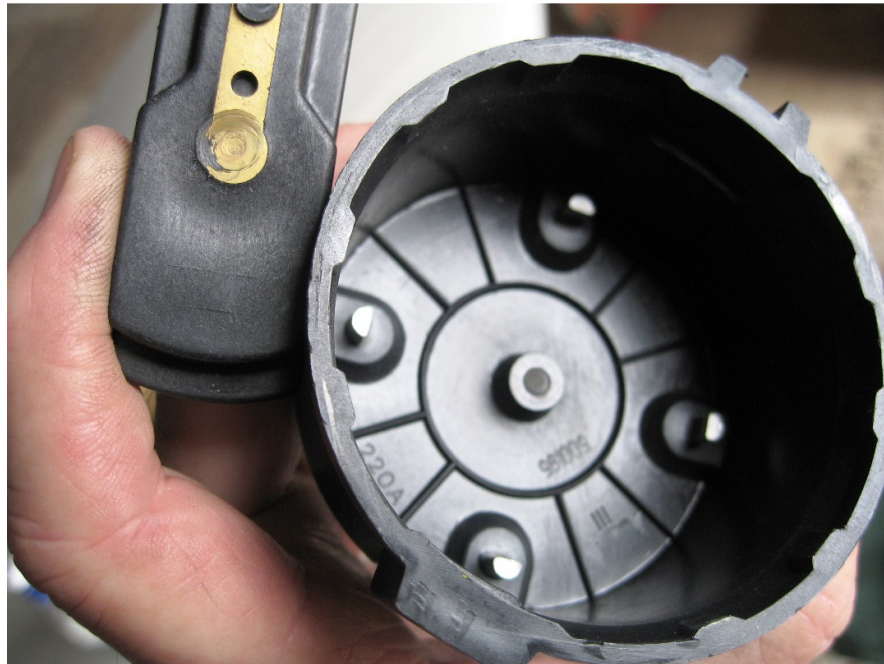
Figure 1 – Damaged Distributor and Rotor
