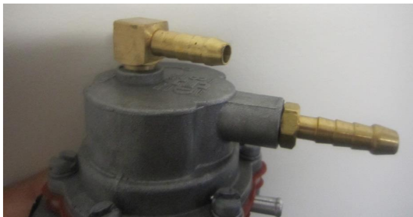
Figure 3: Pump with both fittings screwed in. (No further inspection required)
