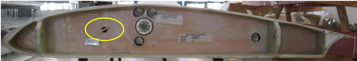
There is a drawstring inside in the wing with extra string coiled around a stick at the aileron end that will be visible through the aileron cable inspection opening. Loosen the drawstring and check that it can be moved freely, then pull a short length out of the wing root (circled above) and tie it firmly through the rod end. Wrap cloth tape around the cable end from the rod end all the way back to the outer cable: this will ease the cable through the wing ribs.
