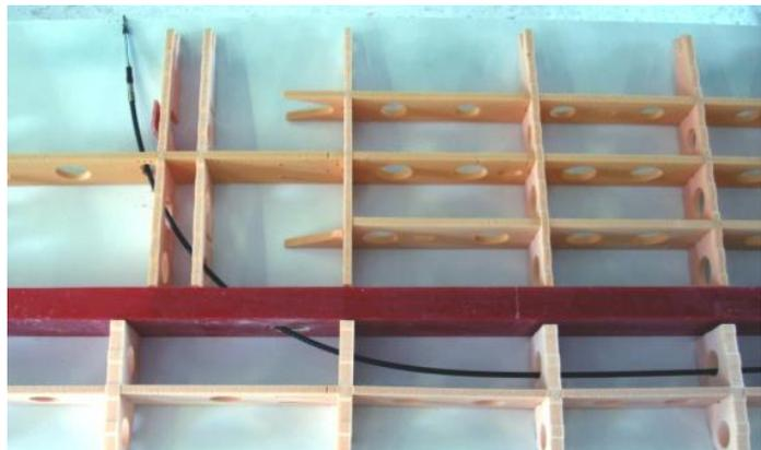
Have your helper feed the cable into the wing while you pull gently on the drawstring through the aileron cable inspection opening. Work slowly and do not apply too much pressure but rather move the cable carefully and shake it if it seems to catch at any time.
